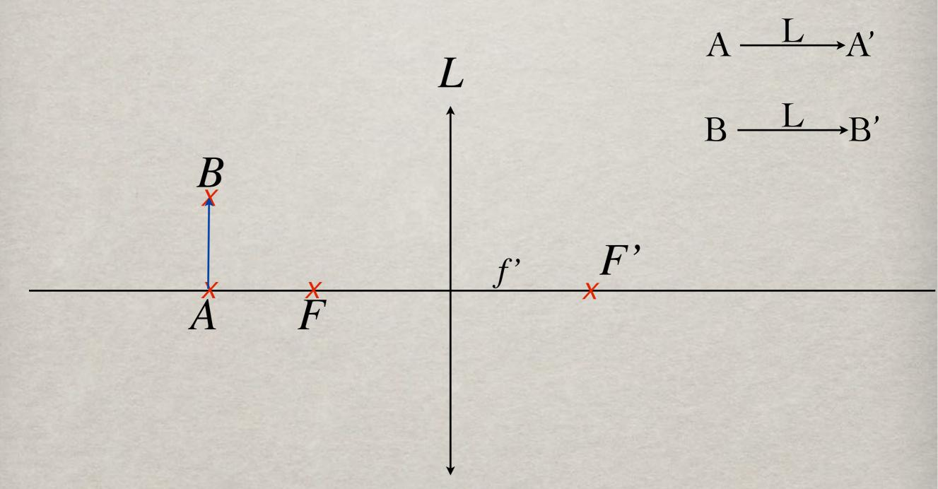
TROIS RAYONS PEUVENT ÊTRE CONSTRUITS POUR DÉTERMINER L'IMAGE [A'B'] DE [AB]
