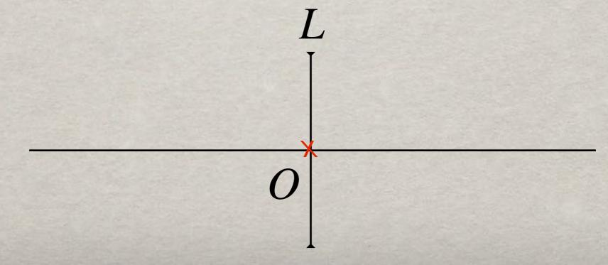
$$\frac{1}{\overline{OA'}} - \frac{1}{\overline{OA}} = (n-1) \left( \frac{1}{\overline{R_1}} - \frac{1}{\overline{R_2}} \right) = \frac{1}{f'}$$
