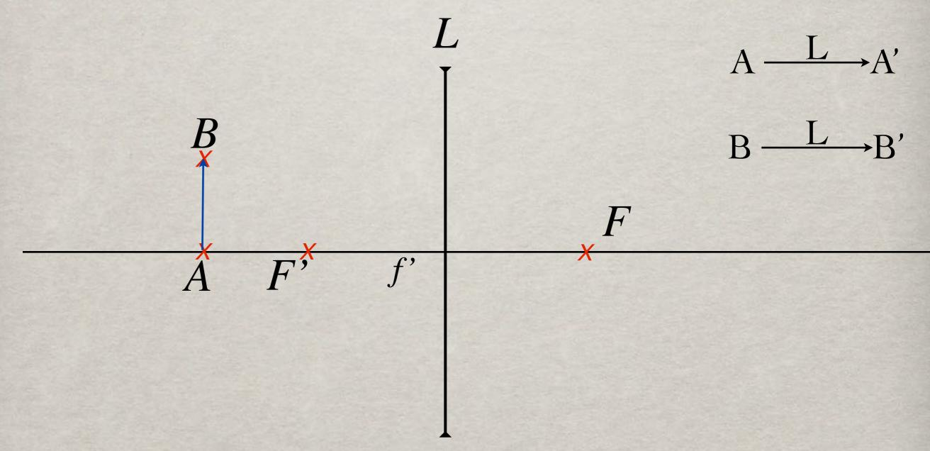
TROIS RAYONS PEUVENT ÊTRE CONSTRUITS POUR DÉTERMINER L'IMAGE [A'B'] DE [AB]
